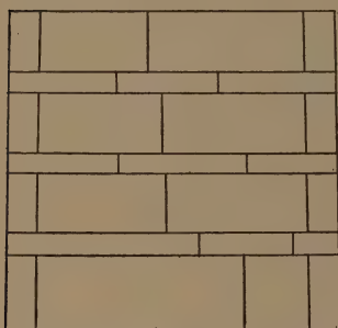
FIG. 14. — Regular, but unequal, coursed masonry from Agrippa Monument, Athens.
